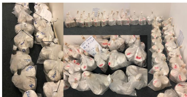
Figure 50. UCS Samples in the 28 Day Curing Period (Border-Tek, 2020)
