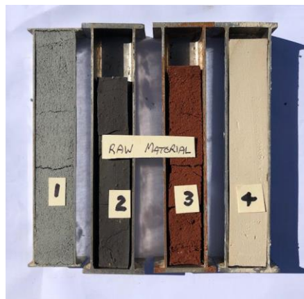
Figure 41. Linear Shrinkage: Raw Materials (Border-Tek, 2020)
