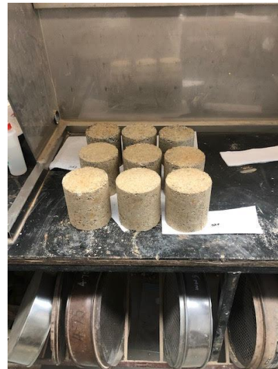
Figure 51. UCS Cast Samples (Border-Tek, 2020)
