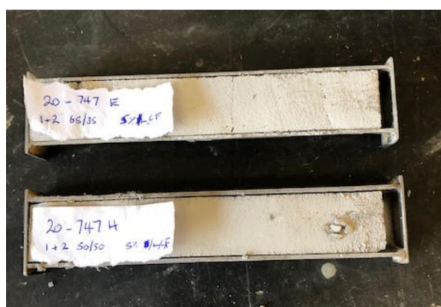
Figure 49. Linear Shrinkage Samples, PT8 (top) and PT9 (bottom) with 5% Lime/Cement/Flyash (Border-Tek, 2020)
