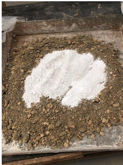
Figure 53. Mixing Slag/Lime Binder with Basegrade Material (Border-Tek, 2020)
