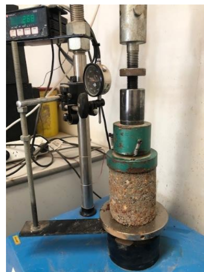
Figure 52. UCS Test Apparatus (Border-Tek, 2020)
