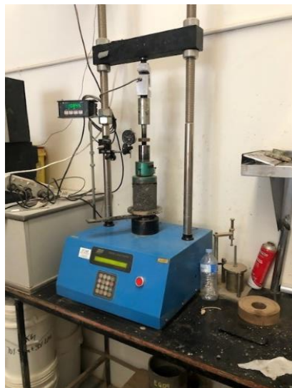
Figure 52. UCS Test Apparatus (Border-Tek, 2020)
