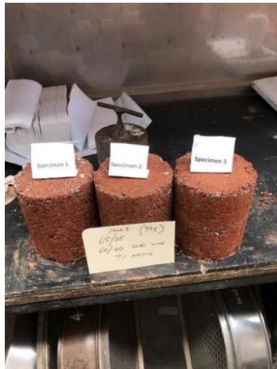
Figure 51. UCS Cast Samples (Border-Tek, 2020)
